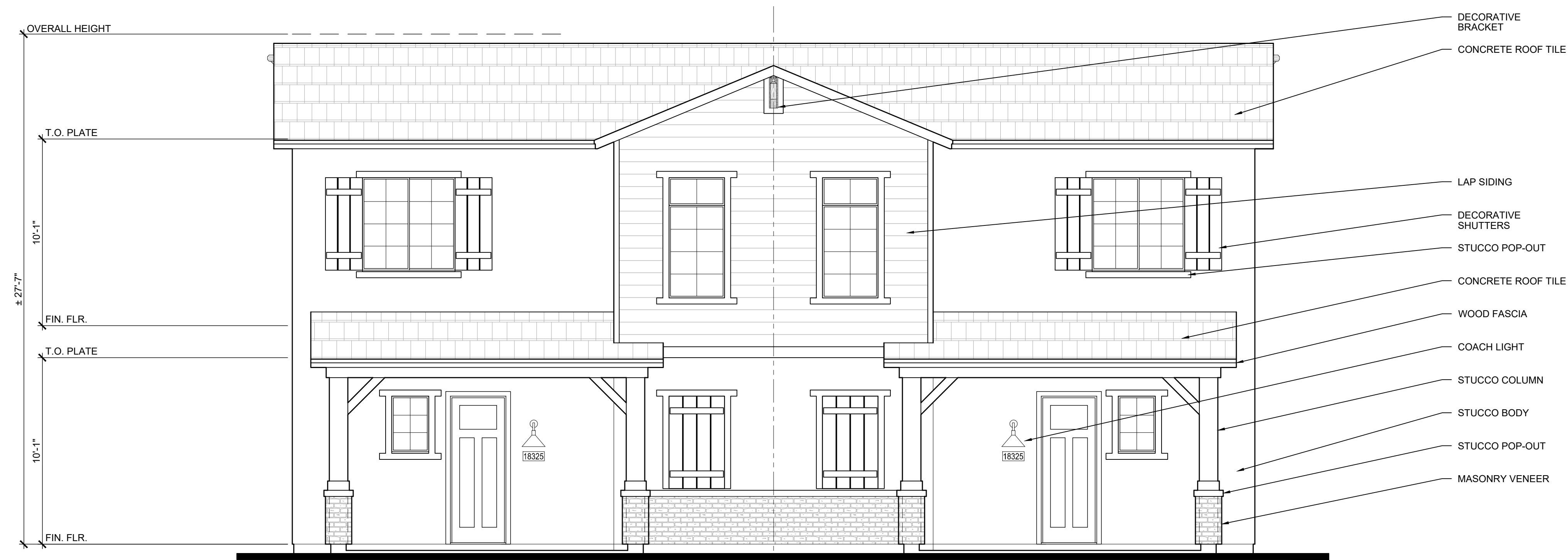
FRONT ELEVATION ELEVATION D - ARIZONA RANCH 1/4" = 1'-0"
