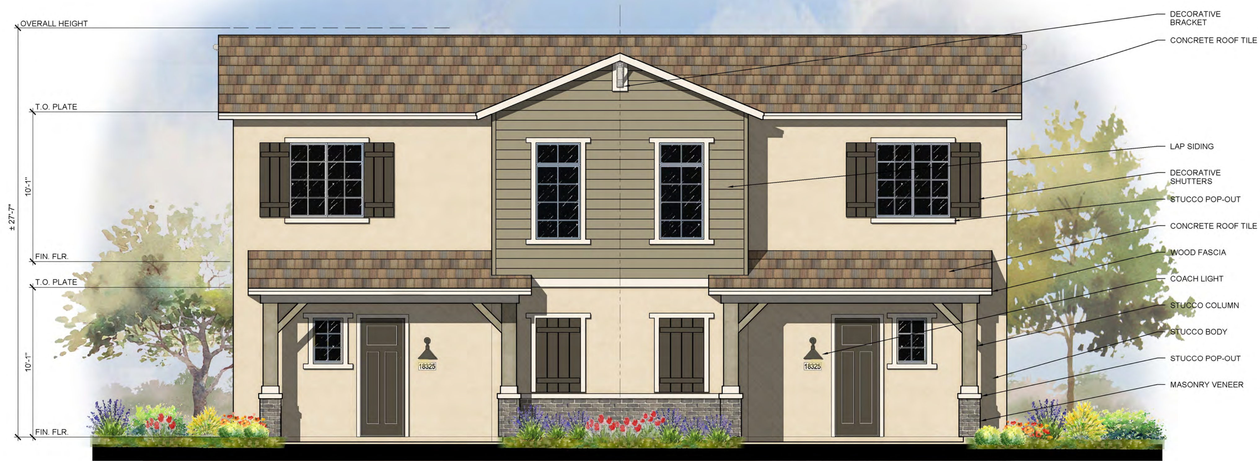
FRONT ELEVATION ELEVATION D - ARIZONA RANCH 1/4" = 1'-0"
