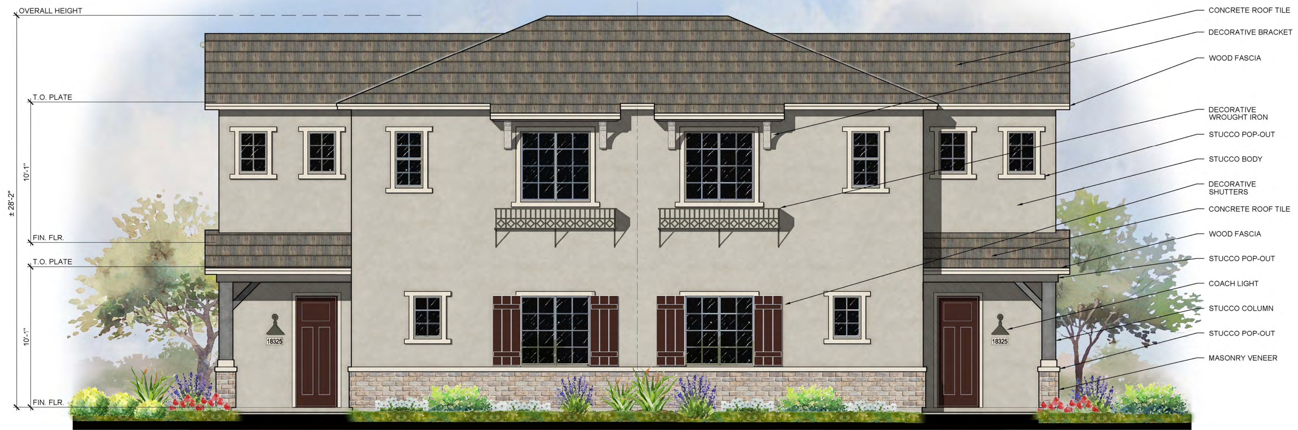
FRONT ELEVATION ELEVATION D - ARIZONA RANCH 1/4" = 1'-0"
