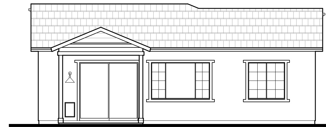
REAR ELEVATION ELEVATION D - ARIZONA RANCH 1/8" = 1'-0"
