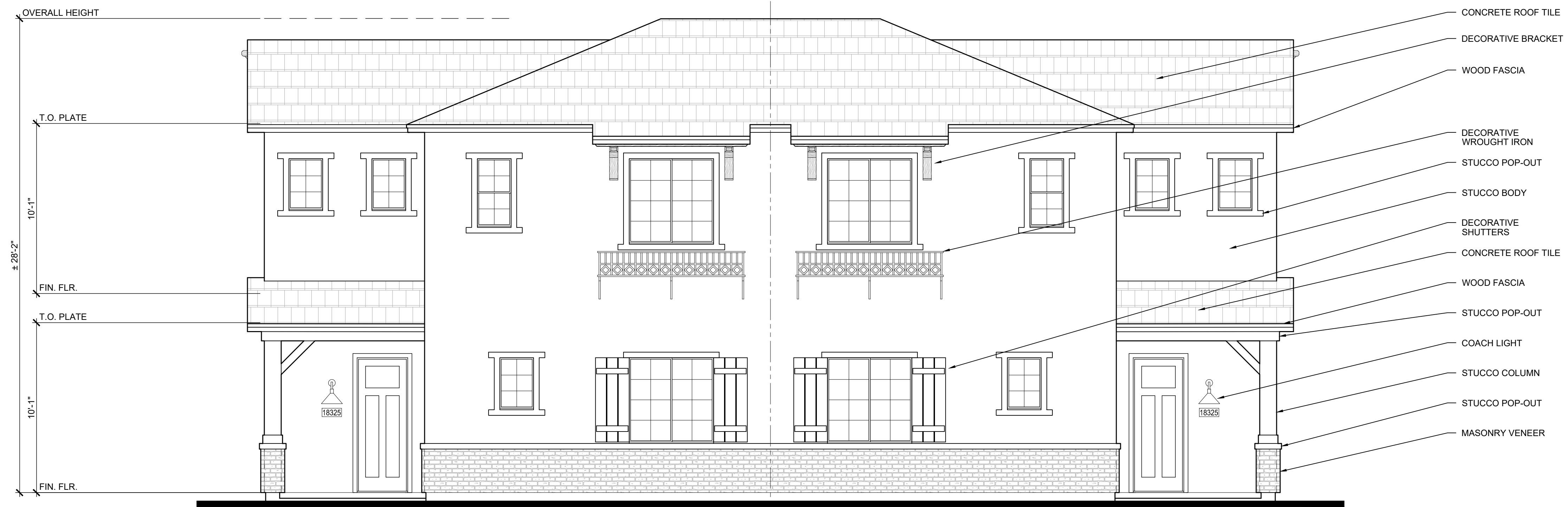
FRONT ELEVATION ELEVATION D - ARIZONA RANCH 1/4" = 1'-0"
