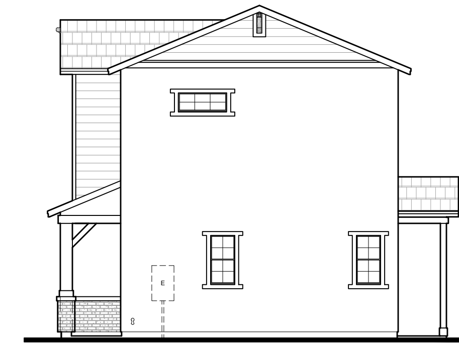
RIGHT ELEVATION ELEVATION D - ARIZONA RANCH 1/8" = 1'-0"
