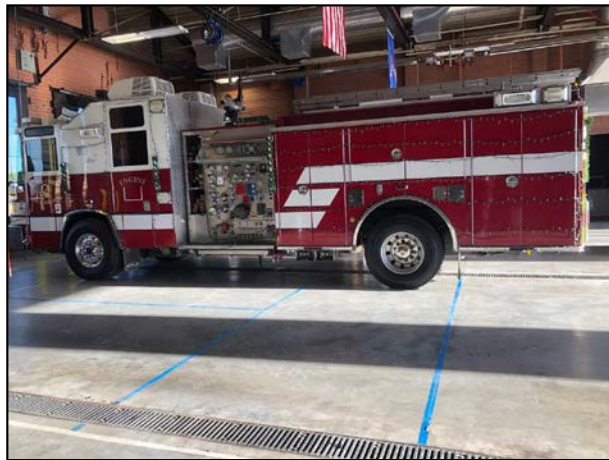
FIGURE 3-10: Reserve Engine (2009 Pierce Quantum Pumper) and Tender 411 (2007 International 7400, 3,000 Gallon Water Tender)
