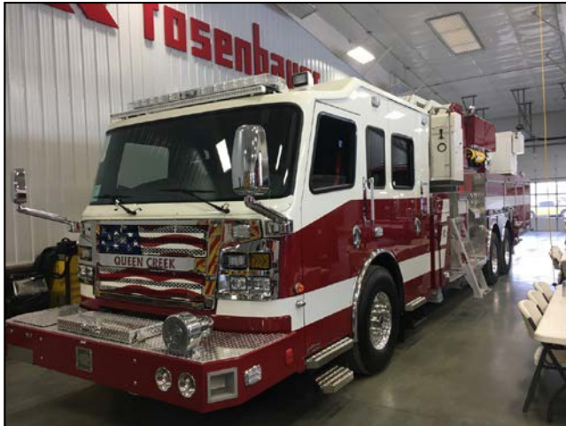
FIGURE 3-13: Ladder 411 (2019 Rosenbauer 88-foot Ladder Tower)
