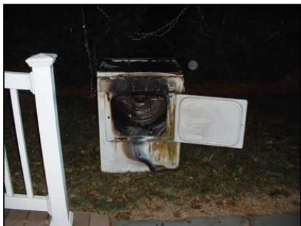
FIGURE 3-26: Clothes Dryer the Only Damage in Sprinkler-Extinguished Fire
