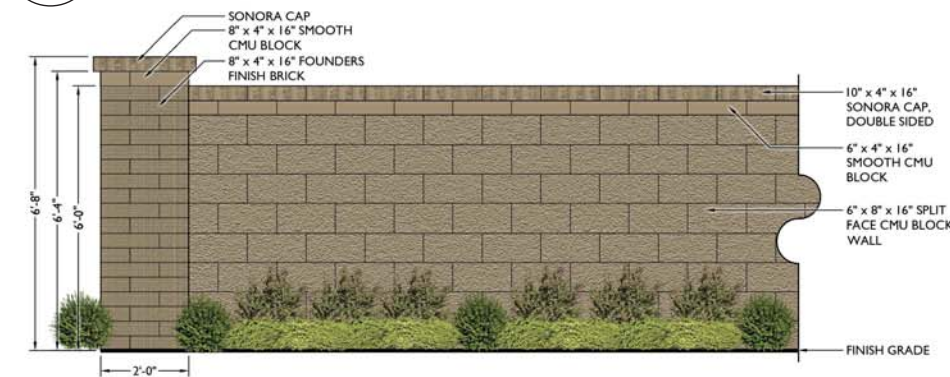
6 DOUBLE SIDED PERIMETER WALL Scale: 1/2" = 1'-0"
