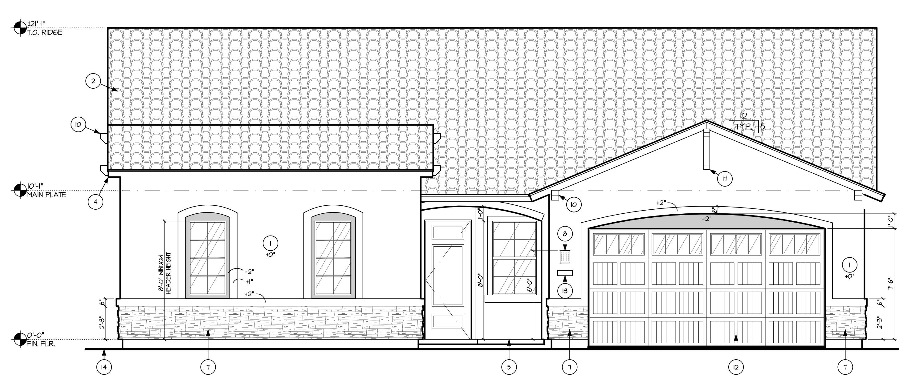
FRONT ELEVATION 'D' SCALE: 1/4" = 1'-0" COTTAGE
