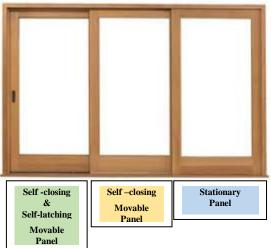
As an alternative, multiple movable panels may be permanently pinned top and bottom to make them stationary and the last moving panel equipped with an approved self-closing device and a self-latching mechanism located at least 54 inches above the floor.
