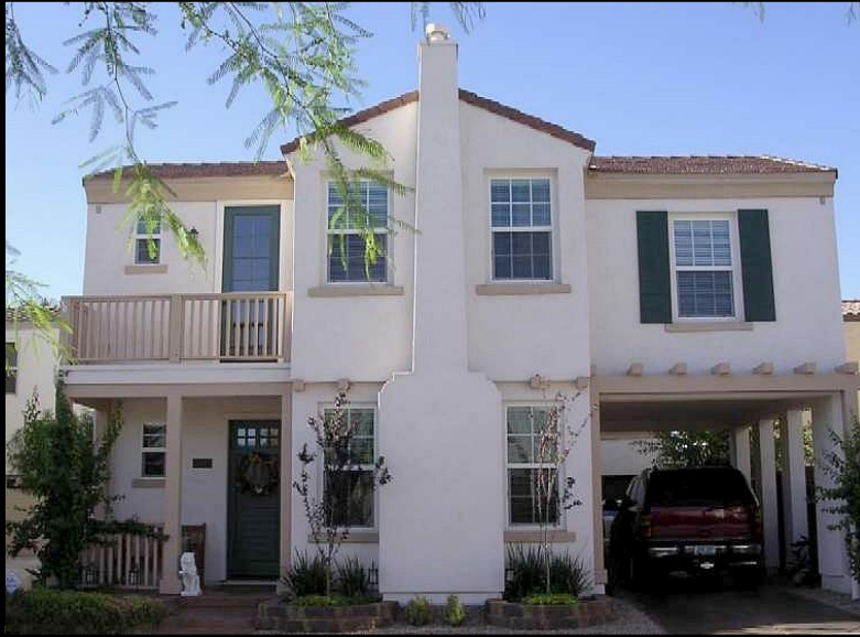
Do This: Windows and doors are aligned and similar in scale creating a sense of proportion and order on this façade.
