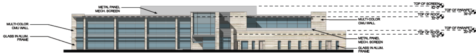
NORTH ELEVATION - PHASE 2
